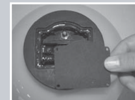
Ensure the seal is positioned correctly
